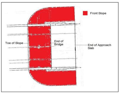
**Figure - Front Slope Definition**
